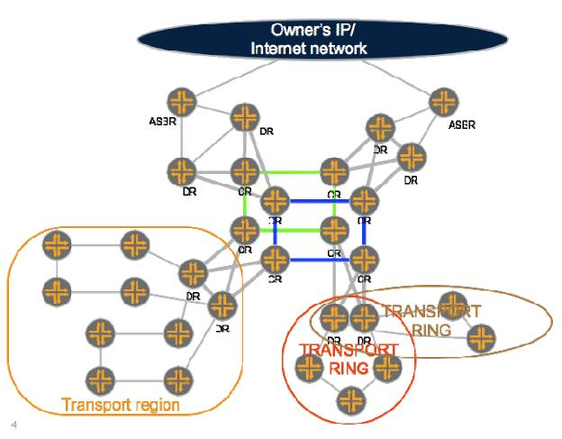
L2 (Eth) DSLAMs are connected to routers on transport rings.
